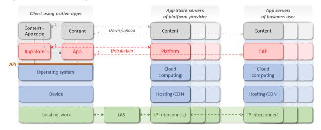
Figure 3 – Provisioning of internet-based services via app architecture
