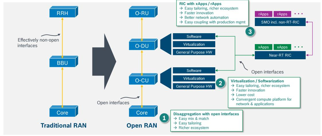
RRH: Remote Radio Head, BBU: Baseband Unit, RAN: Radio Access Network, RU: Radio Unit, DU: Distributed Unit, CU: Centralized Unit, RIC: RAN Intelligent Controller, SMO: Service Management & Orchestration, RT: Real-Time
