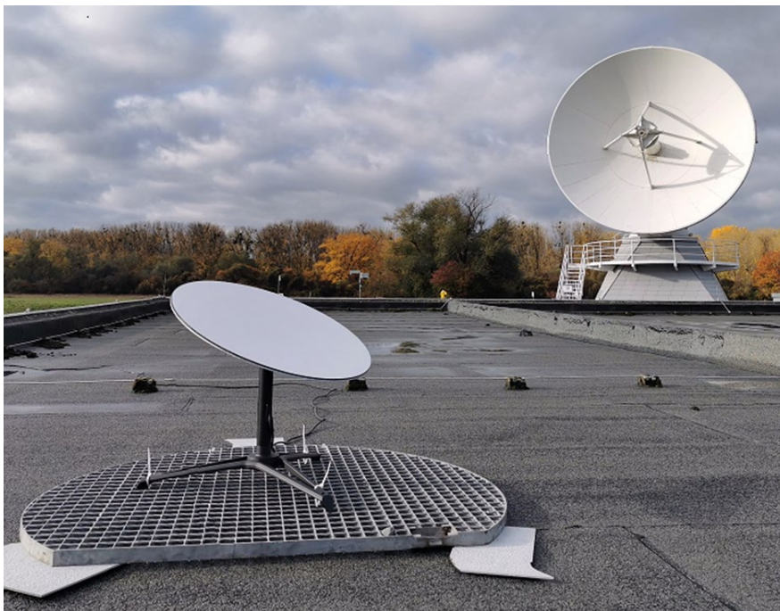
Figure 3: StarLink Terminal 50 cm (at Leeheim Satellite monitoring station of the Federal Network Agency in Germany, measured performance: DL: 100 Mbit/s, UL: 25 Mbit/s, latency: 44 ms typical)
