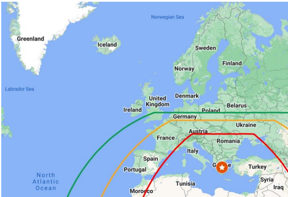
mPOWER coverage areas: Green is with 11 MEOs (2025), Orange with 8 MEOs (2023) and Red with 6 MEOs (Q1 2023)
